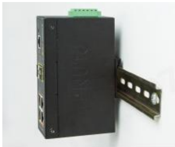
Figure 6-26 DIN Rail Installation
